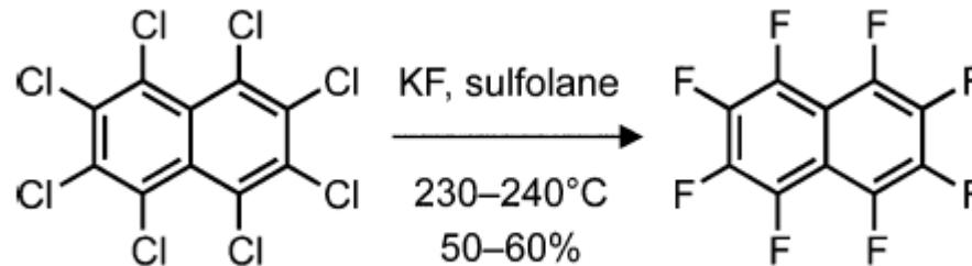
Nucleophilic aromatic substitution of electron-poor arenes (the Halex process).
