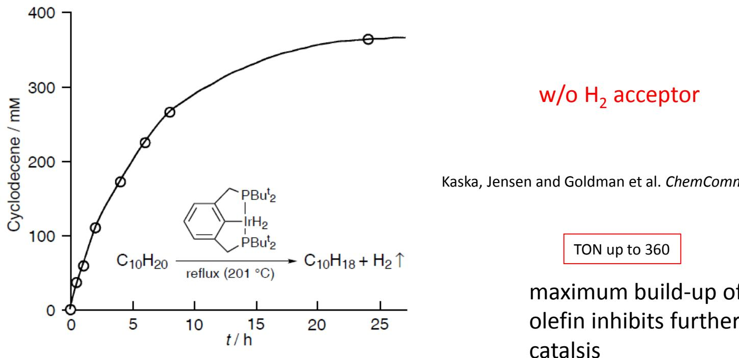
**Fig. 1** Cyclodecene formation (total, ca. 3 : 1 *cis:trans*) vs. time; (PCP)IrH<sub>2</sub> in refluxing cyclodecane (1.0 mM, 201 °C)
