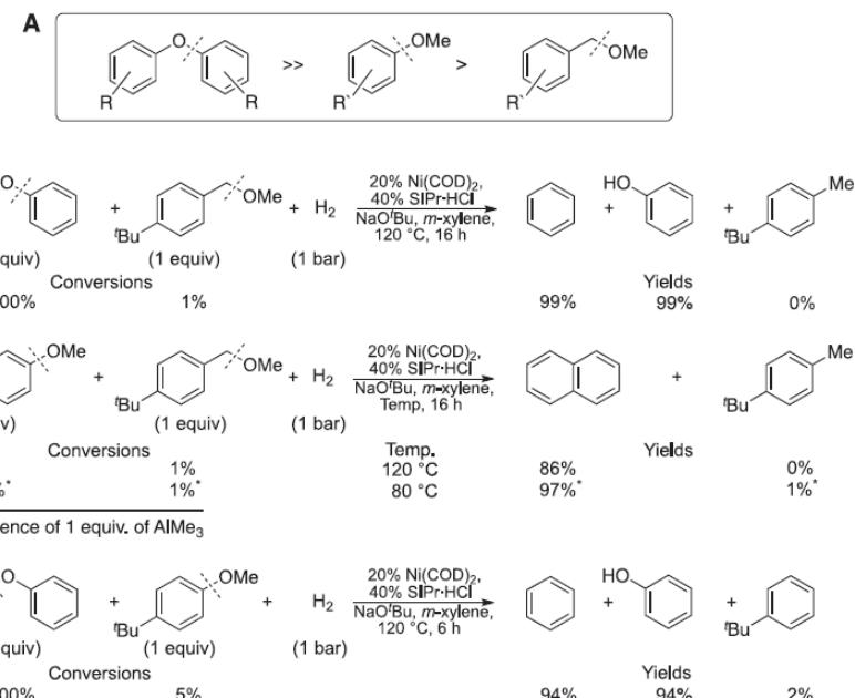
**Fig. 2.** (A) Relative reactivity of aryl and benzyl ethers toward hydrogenolysis of C–O bonds catalyzed by Ni(COD)<sub>2</sub> and SiPr. Selective hydrogenolysis of (B) diphenyl ether in the presence of 4-*tert*-butylbenzyl methyl ether; (C) 2-methoxynaphthalene in the presence of 4-*tert*-butylbenzyl methyl ether; and (D) diphenyl ether in the presence of 4-*tert*-butylanisole.
