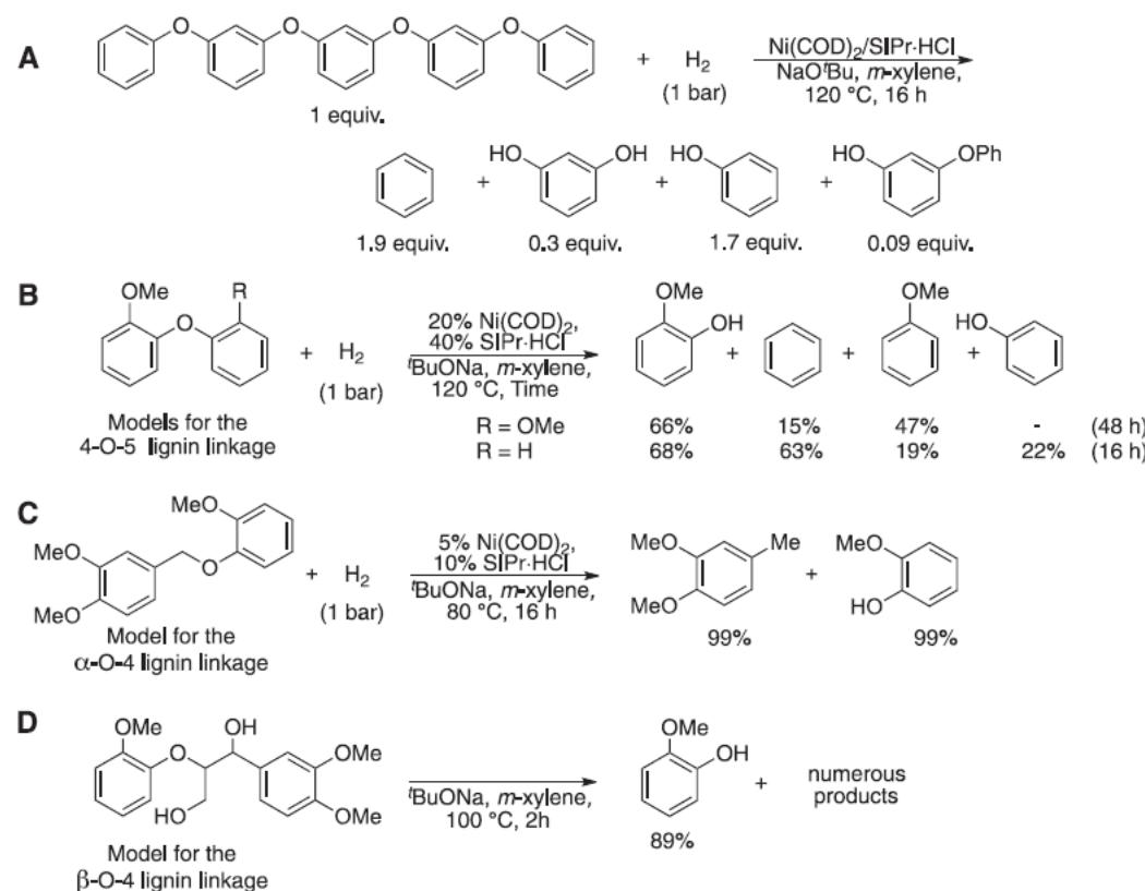
**Fig. 3.** Hydrogenolysis of (A) bis(*m*-phenoxyphenyl)benzene. (B) A model of the 4-O-5 linkage in lignin. (C) A model of the  $\alpha$ -O-4 linkage in lignin. (D) A model of the  $\beta$ -O-4 linkage in lignin.
